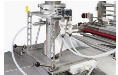
Hose station for cleaning
