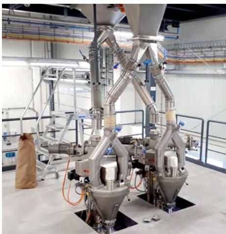
**Both paper bags and plastic bags can be produced on the SBS Twin from ROVEMA**, at Bauck in formats from 250 grams to 1-kilogram bags. Before the oat flakes fall into the bags, they are transported directly from the silo to the auger feeder by means of a pipe chain conveyor. According to Stahl, this is a special feature, as flakes are often dosed with multi-head weighers.
