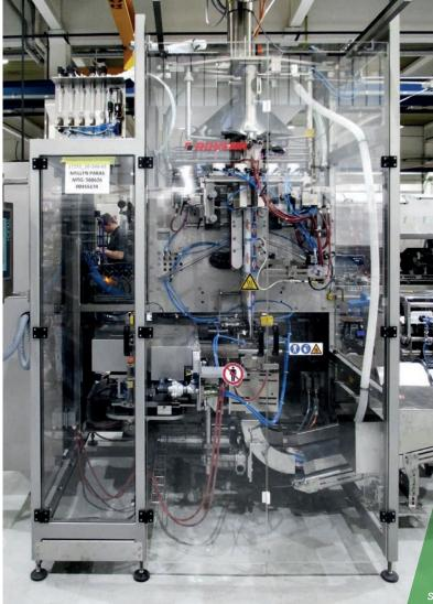
One of two new VPI 400 with swiveling cross sealing station at the Fernwald plant.
